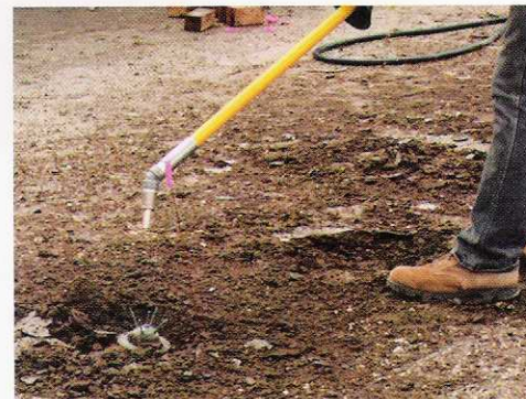
The specially designed air nozzle creates a focused jet of air at Mach 1.5 speed for easy mine excavation.
