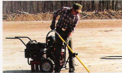
Compared to current digging practices, the Air Spade reduces operator fatigue and back strain, and the air tool provides a safer standoff for deminers.
