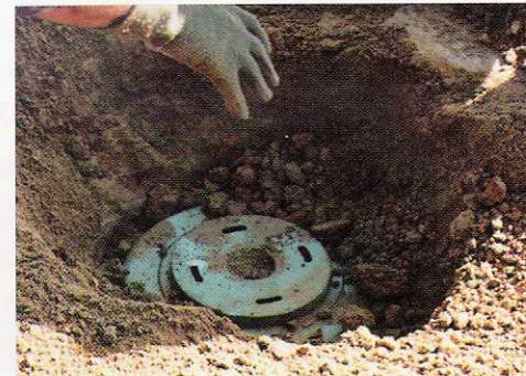
The Air Spade is especially useful against deep buried mines in dry hardpacked soil.
