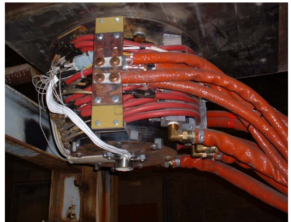
Prototype MAG-GATE™ device mounted to bottom of test tundish
