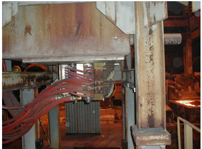
Prototype MAG-GATE™ device mounted to bottom of test tundish
